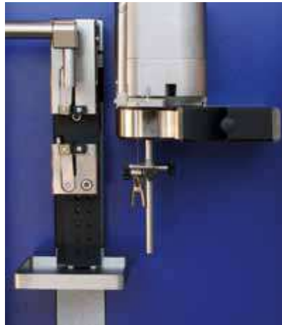
Fiber transfer from the vibroscopic measuring head to the tensile test section
