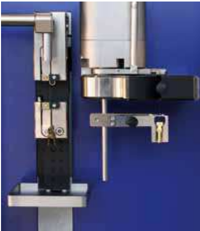
Fiber transfer from the vibroscopic measuring head to the tensile test section
