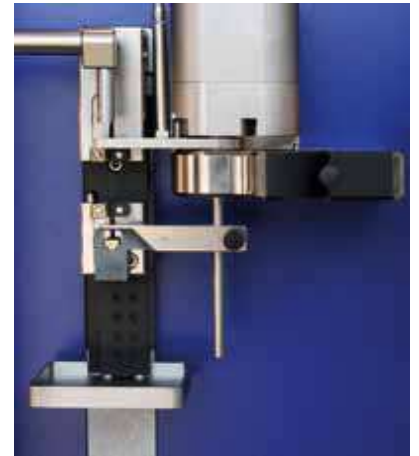
Fiber transfer from the vibroscopic measuring head to the tensile test section
