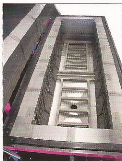
Cleaning chamber of VACUCLEAN 254
